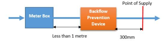
When the separate backflow prevention device is further than one metre from the meter box
